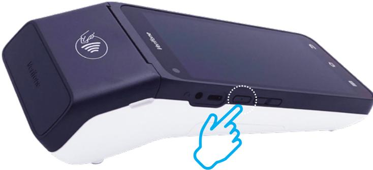
Press the power button on the side of the terminal.
