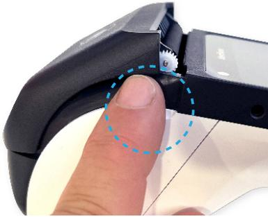
Open paper roll cover of the T650c as shown above. There are small slots to aid opening if required
