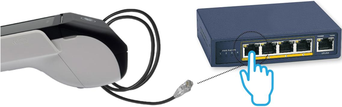
Plug the other end of the Ethernet cable into a free LAN port on your router. Look for the Ethernet icon
