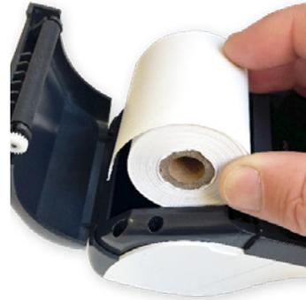
Remove used paper roll. Insert new roll so the paper feeds from the top, leaving a length of paper sticking out of the terminal
